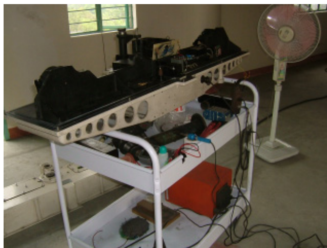
Photo. 3 Repair and checks of Dobson in penthouse.
