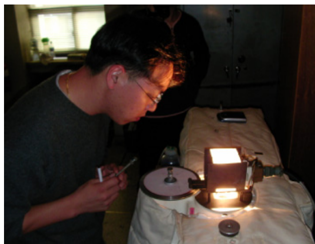
Photo. 3 Thickness inspection of the optical wedge using the repaired two lamp check equipment.
