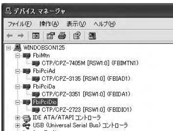
Fig. 10 Status of I/O modules by Windows device manager.
