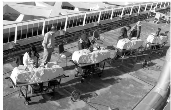
Photo. 3 Total ozone intercomparison observation was performed under expert's guidance. (Instruments are the Philippines, Thailand, India, and Asia regional standard Dobson from left-hand side).
